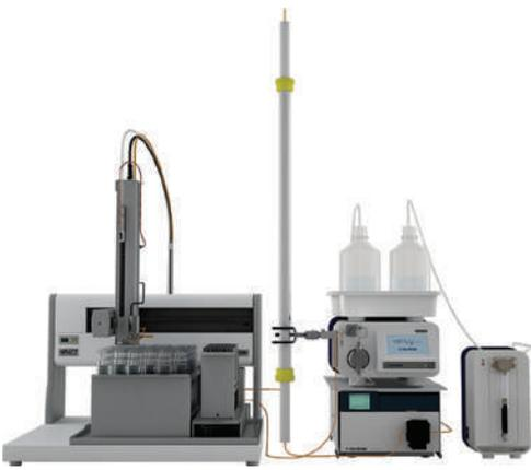
**AUTOMATED GPC CLEANUP FOR A VARIETY OF SUBSTANCES, MONITORED BY UV DETECTION**
