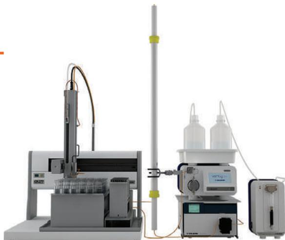
The VERITY<sup>®</sup> GPC Cleanup System is configured with a GX-271 Liquid Handler equipped with 3-ways collection valve, GX Direct Injection Module, VERITY<sup>®</sup> 4020 Single Syringe Pump, VERITY<sup>®</sup> 3011 Isocratic Pump, TRILUTION<sup>®</sup> LC Software, and an optional 157 UV-VIS Detector
